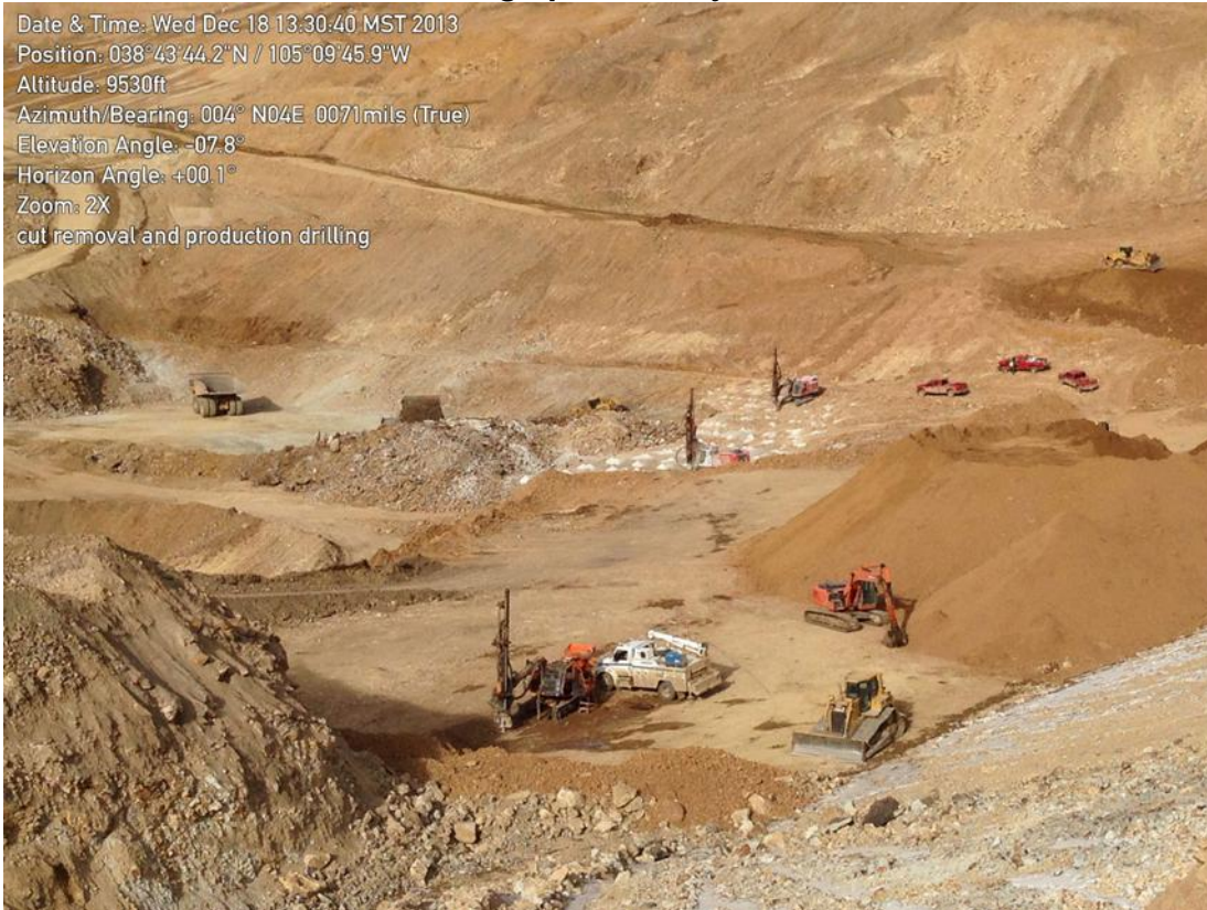
Photo 1: Cut removal and production drilling along Bench A.
