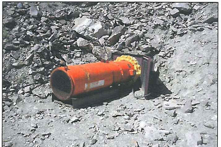
Vent fan installed in culvert at 9700 portal
