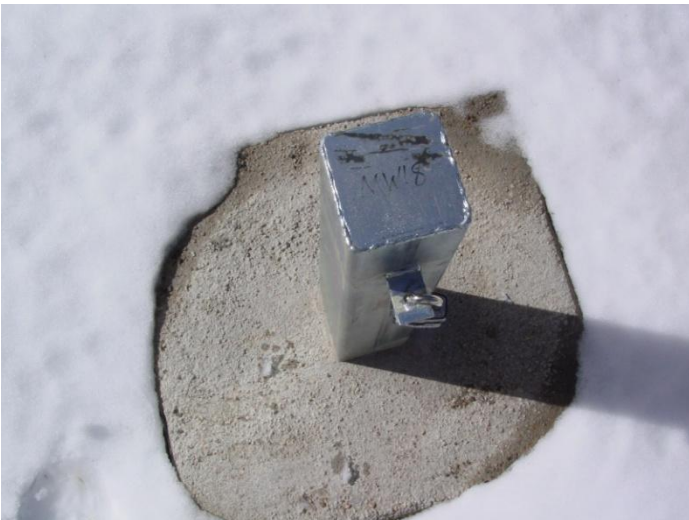
Photo 5 – Wellhead of new bedrock ground water monitoring well MW-18 (screened interval 215 – 235 ft in Illinois Fault well near Sump 10).
