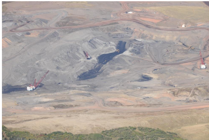
Active mine area, draglines on the left mining in L and M pit. Dragline on the right staged near scoria pile.
