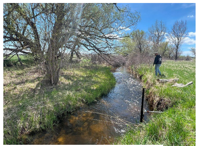
Figure 2 Hydrographers building a natural streamgage control South Boulder Creek above Howard Ditch
