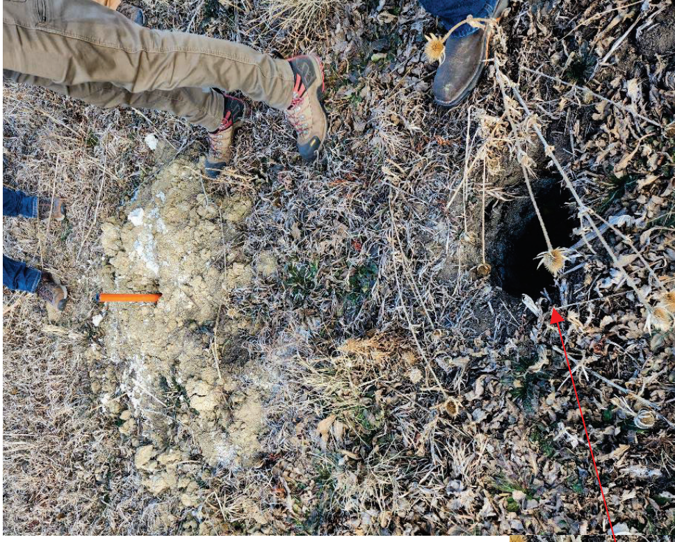
Photo 6 - Boring backfill and drill outrigger pad
