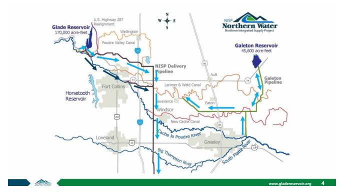
Glade Reservoir (top left corner in image above) would store 170,000 acre-feet of water and have a surface area of approximately 1,600 acres at full capacity. Seven miles of Highway 287 will be relocated east.
