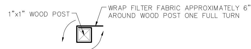
1. WRAP APPROXIMATELY 6" OF FILTER FABRIC OF EACH END AROUND A WOODEN POST ONE FULL TURN, THEN SECURED ALONG THE POST WITH HEAVY DUTY WIRE STAPLES AT LEAST 1" LONG. 2. POST SHALL BE TIGHTLY ABUTTED WITH NO GAPS TO PREVENT POTENTIAL FLOW-THROUGH OF SEDIMENT AT JOINT.
