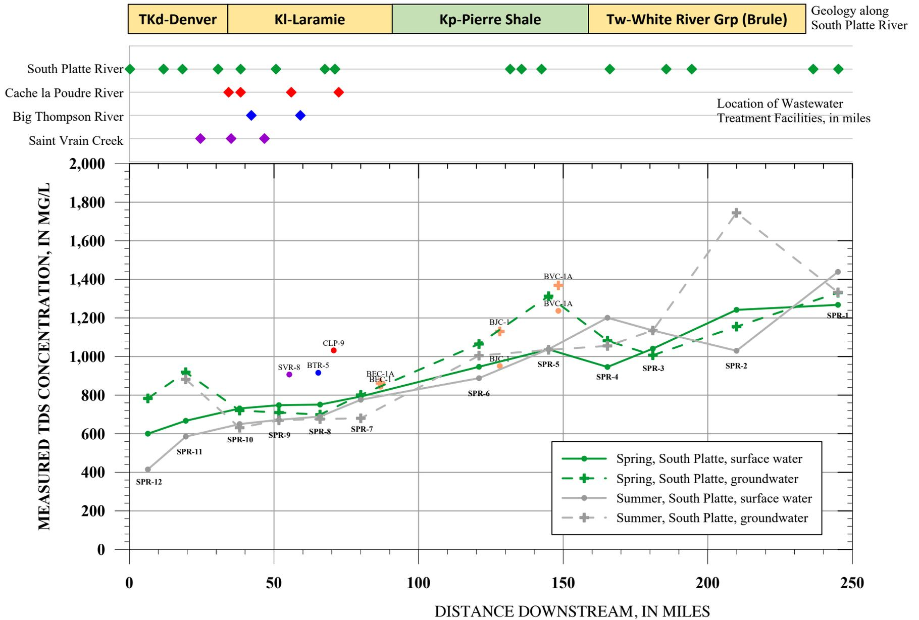
**Figure B-1-1. Total Dissolved Solids concentrations along the South Platte River**
