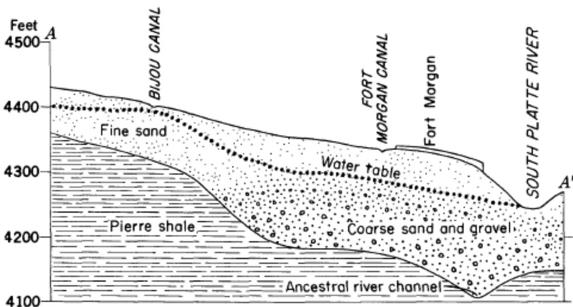
Figure 4-2. Map and section showing groundwater flow to the South Platte River (Bjorklund and Brown, 1957)
