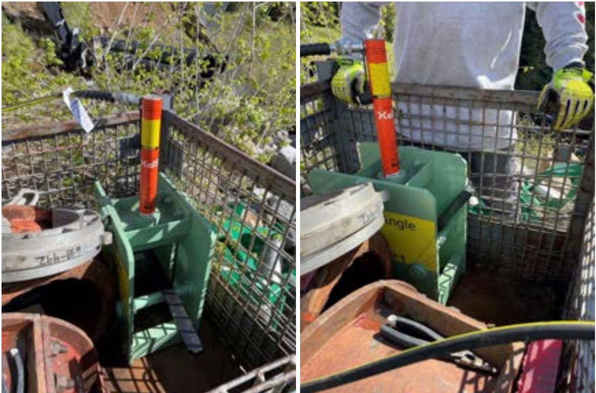
Photos 15 & 16: Performing reverse back bend test. Hydraulic press used to bend HDPE test section to 120°.
