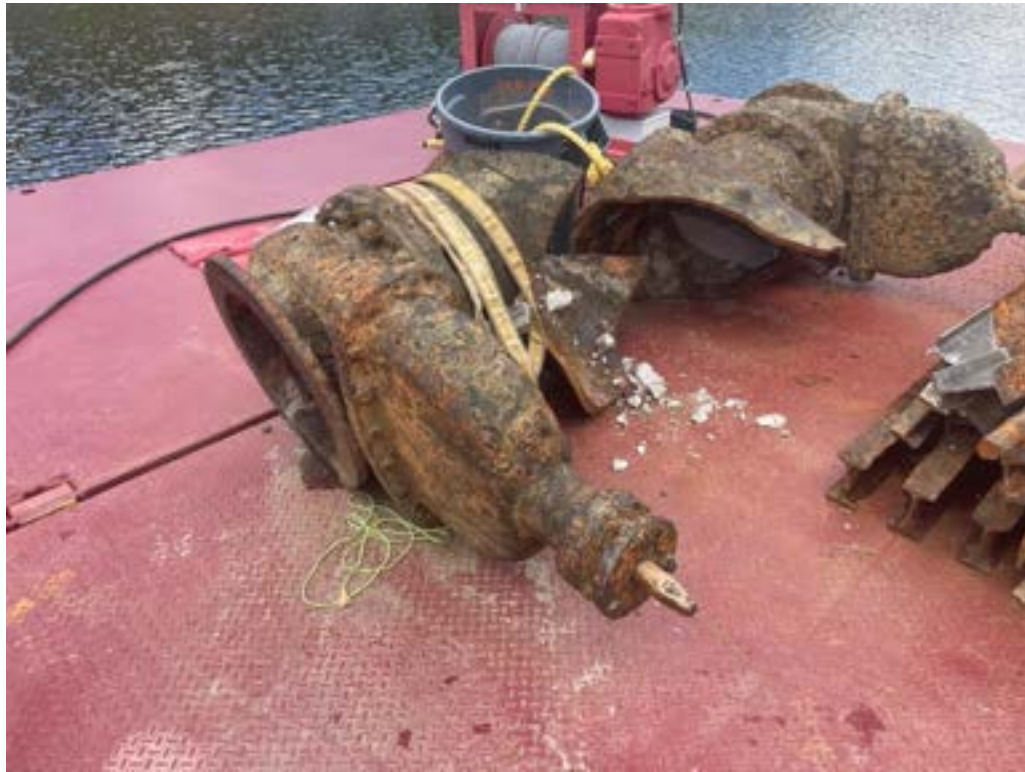
Photo 12: Right side of tee and gate broken off and removed from structure.
