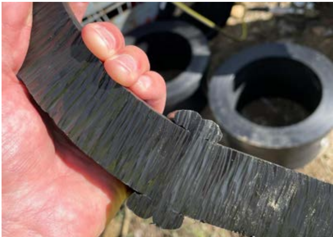
Photo 17: Result of reverse back bend test. Weld is shown to be intact and free of defects. Test was performed on four separate test sections with same result.
