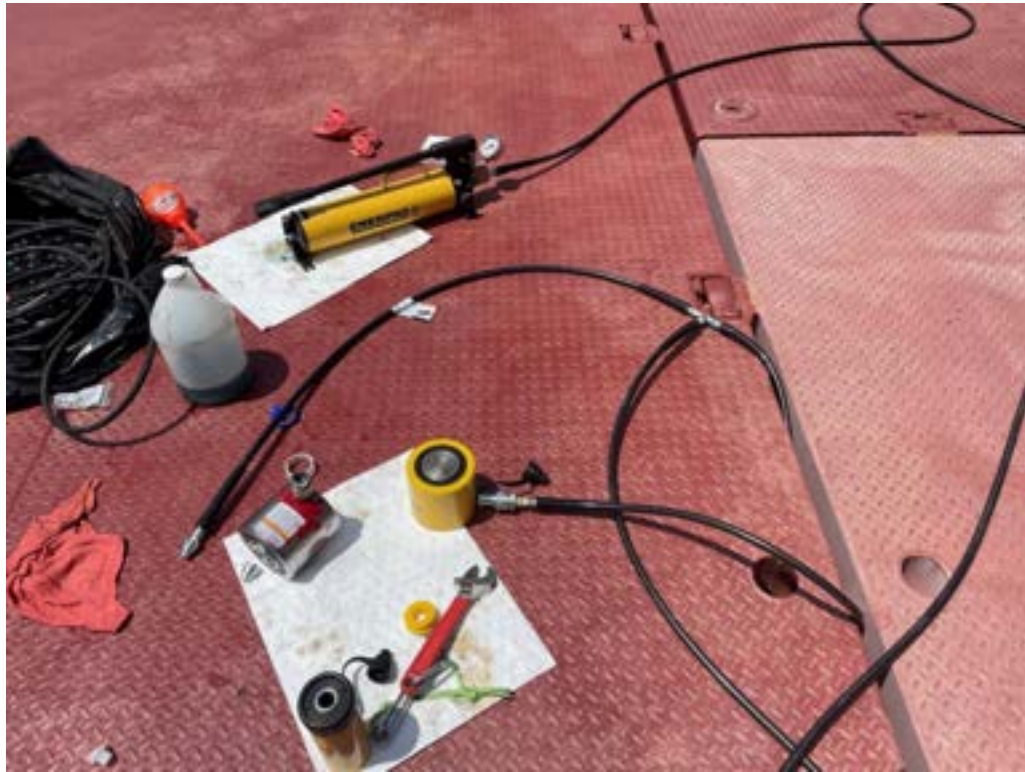
Photo 3: Hydraulic pump and ram with 2-inch stroke.
