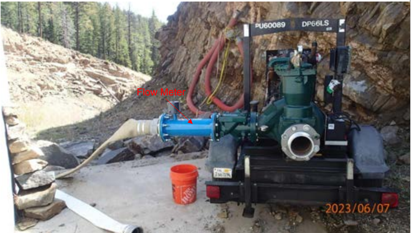
Photo 6: 6-inch trash pump setup with inline flow meter.
