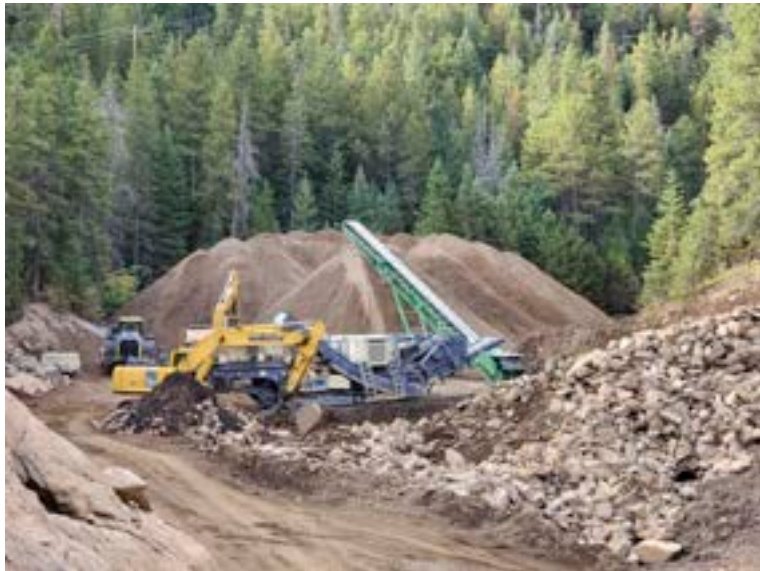
Rock crusher on site making RCC material from old dam rubble
