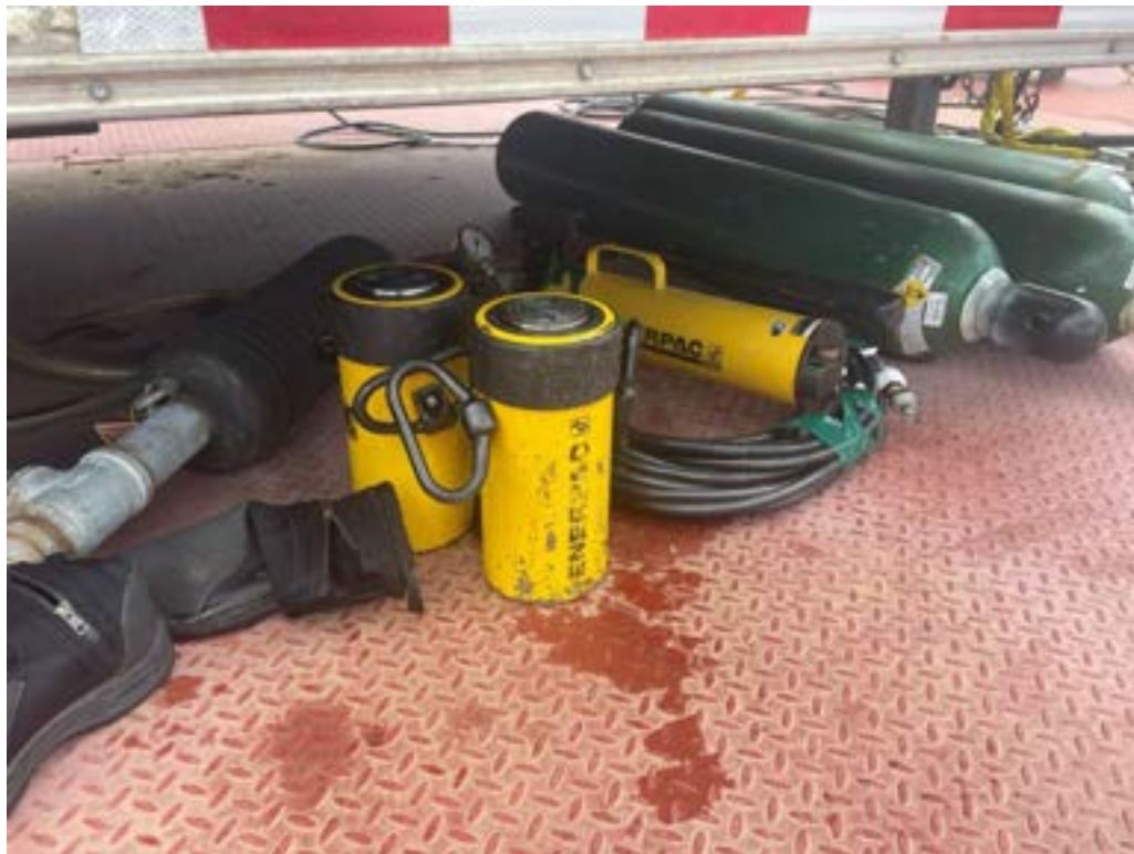
Photo 4: Hydraulic rams with 6-inch stroke
