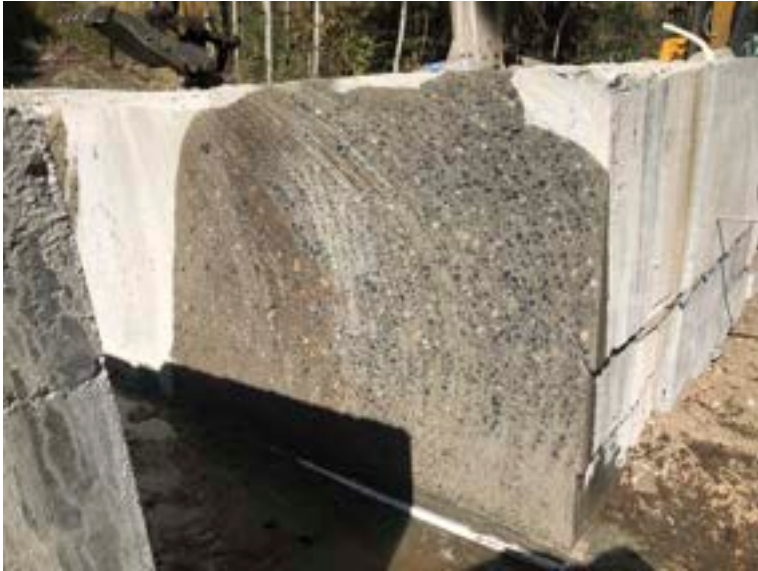
Test patch is cut to be evaluated by engineers, it was good to go
