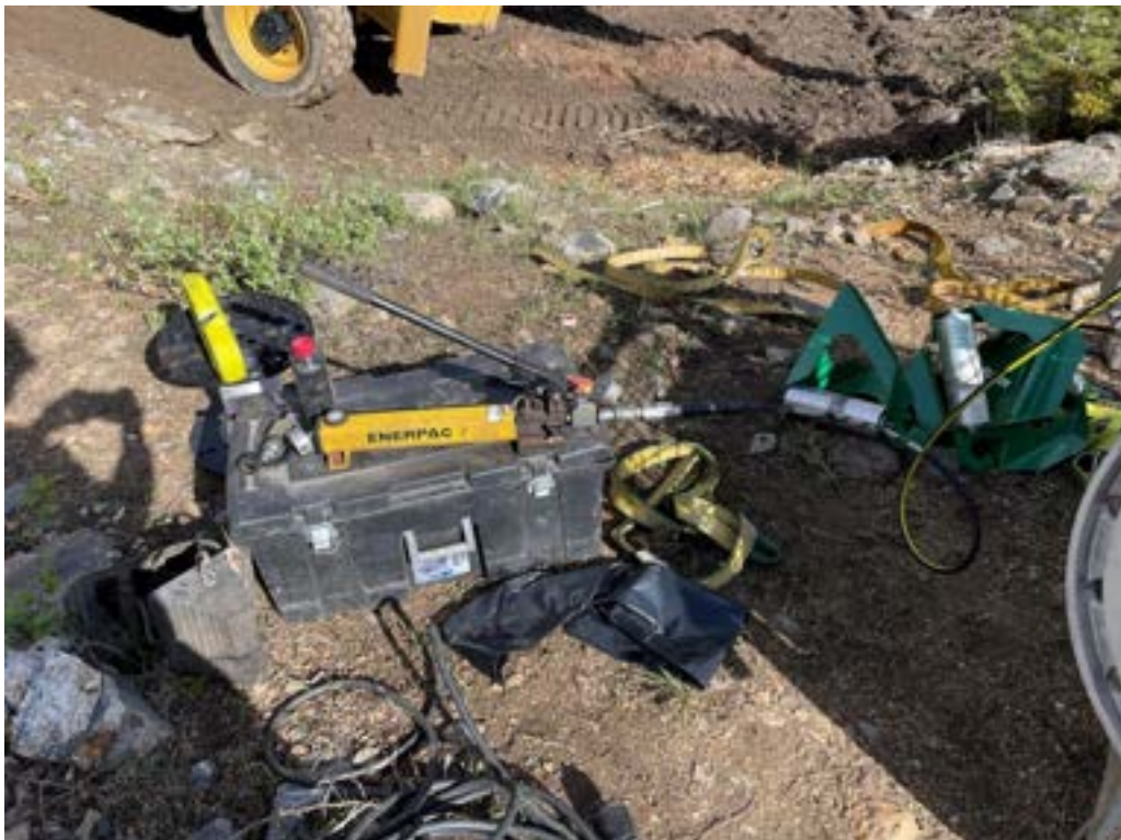
Photo 14: Hydraulic press used to perform reverse back-bend test on HDPE test weld.
