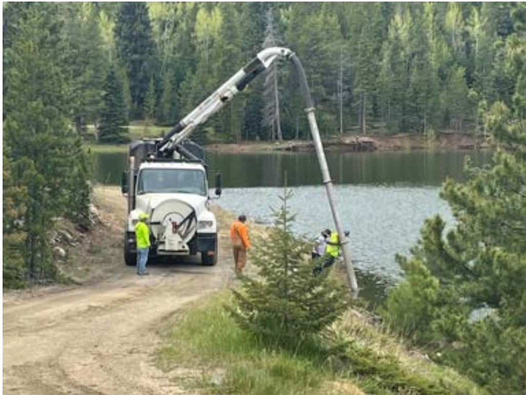
Photo 24: Vac truck used to collect water for jetting operations. 600-ft hose reel is affixed to front of vac truck.
