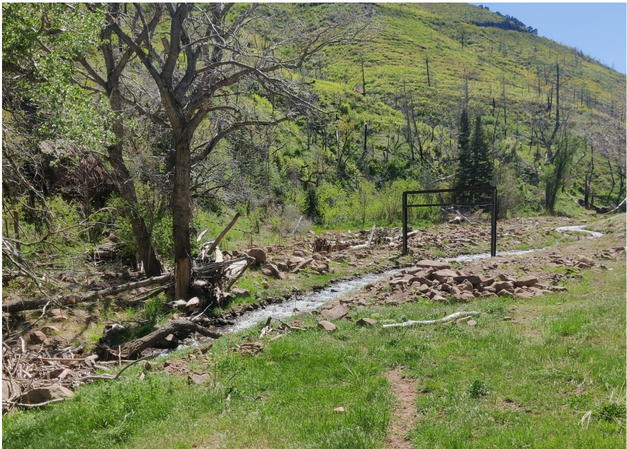
Completed Middle Creek flood warning gage site; gage mounted on metal frame shown (center right)
