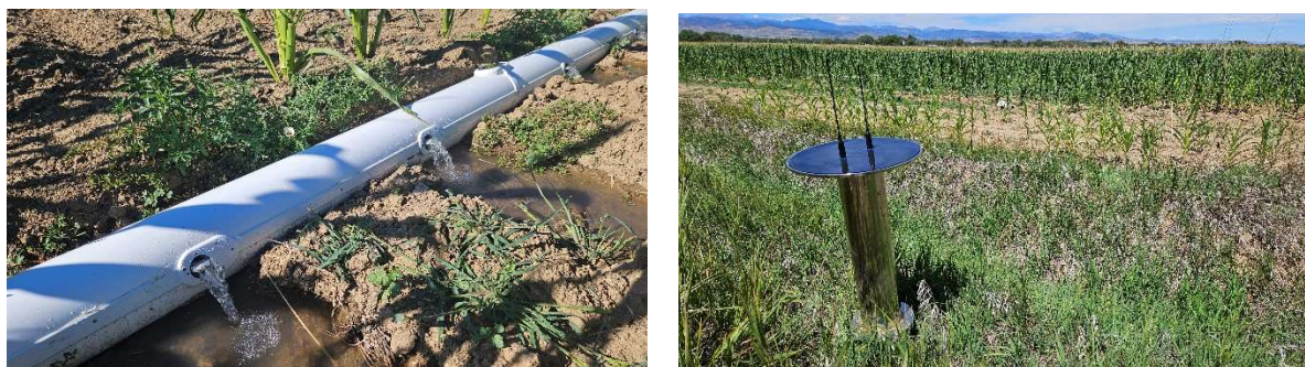
Figure 4 Pre-assembled pipe in operation (left), with field controller radio unit (right)
