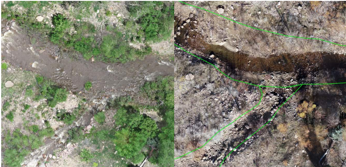
Figure 3. UAS imagery taken during high flows (left) used to delineate active stream channel during low flows (right). Green lines show the final stream channel delineation.
