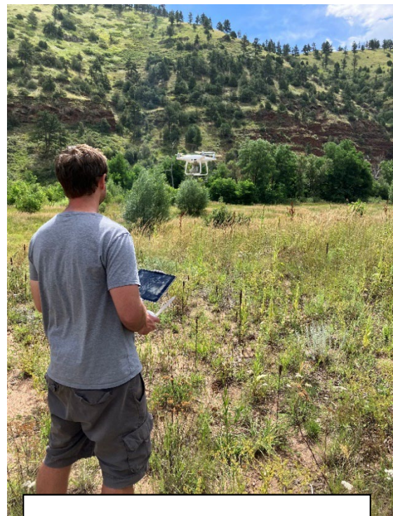
A UAS (i.e., drone) takes off to collect static images that are used to develop digital elevation models
