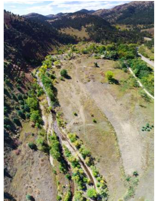
Downstream Reach: traditional restoration site with uniform floodplain grading and limited features.
