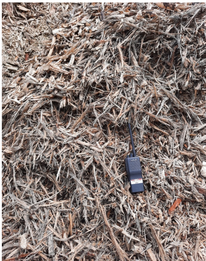
Figure 7. Quality and size of wood shred at Landing 3.
