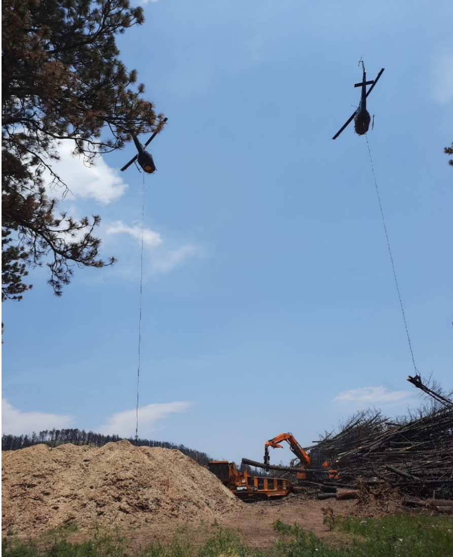
Dueling helicopters at Landing 4 on the Cal-Wood Education Center. When and where feasible, one helicopter would transport logs to a landing for processing while another simultaneously flew mulch onto hillslopes.
