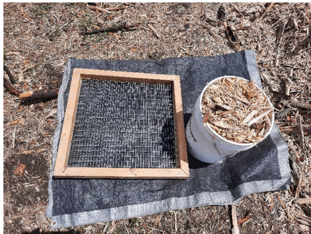
Figure 6. Screen for wood shred mulch quality control.
