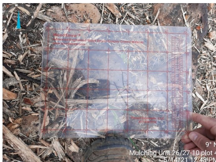
Figure 9. Mulch coverage monitoring grid (Forest Concepts LLC, Auburn, WA).
