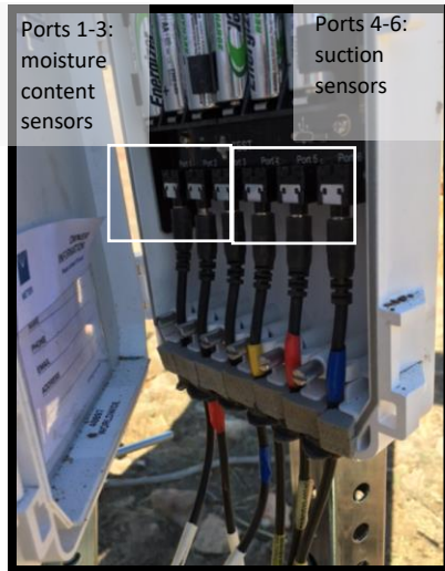
Detail of connections to datalogger (Figure 4), Schematic of subsurface instrumentation (Figure 5)
