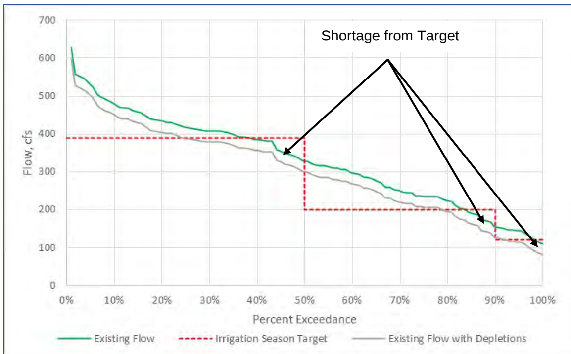
Figure 8-3: Flow Duration Curve for Forecast Year 2017 Irrigation Season (Average Hydrologic Year)
