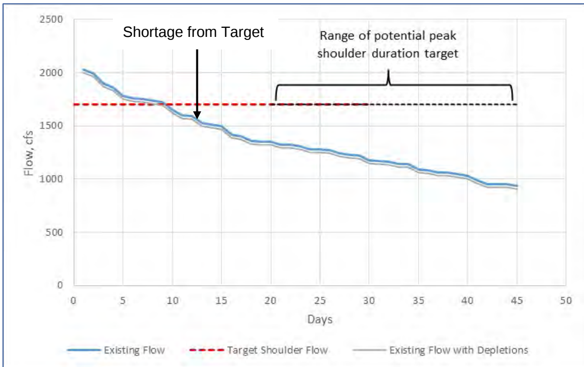
Figure 8-5: Shoulder Flow Magnitudes and Durations for Forecast Year 2017 (Average Hydrologic Year)
