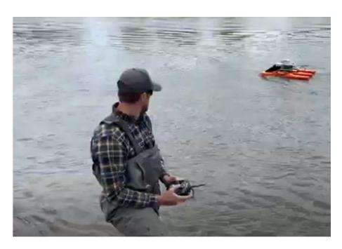
Remote-controlled Automatic Data Collection Platform (ADCP) system developed by DWR to expand use and improve safety of ADCP's
