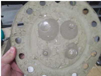
200 mils with mesh reinforcement 1" hole failure at 2200 psi
