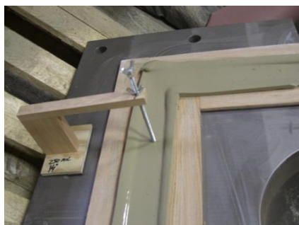
QC tool to ensure proper seal install
