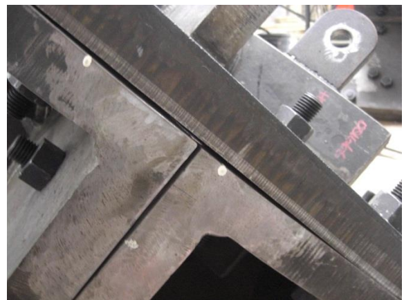
Notice the increase in the gap of the fixture under Pressure for 63 days without compromise of the seal
