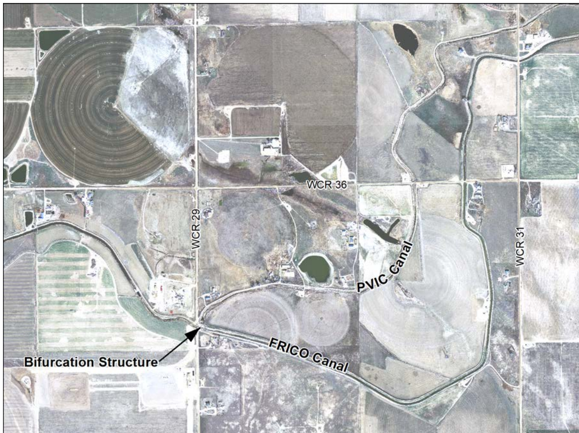
Figure 1. Equalization Reservoir Bifurcation Structure Location Map.
