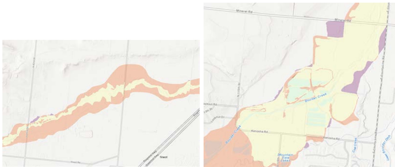
Figure 11. Left: Left Hand Creek FHZ versus Floodway, with some very small segments where the FHZ has a smaller extent (purple areas show presence of Floodway only, red is FHZ only, and yellow is both FHZ and Floodway coverage). Right: Boulder Creek near Erie, with FHZ and Floodway having some inconsistency but the FHZ extent still appearing reasonable.
