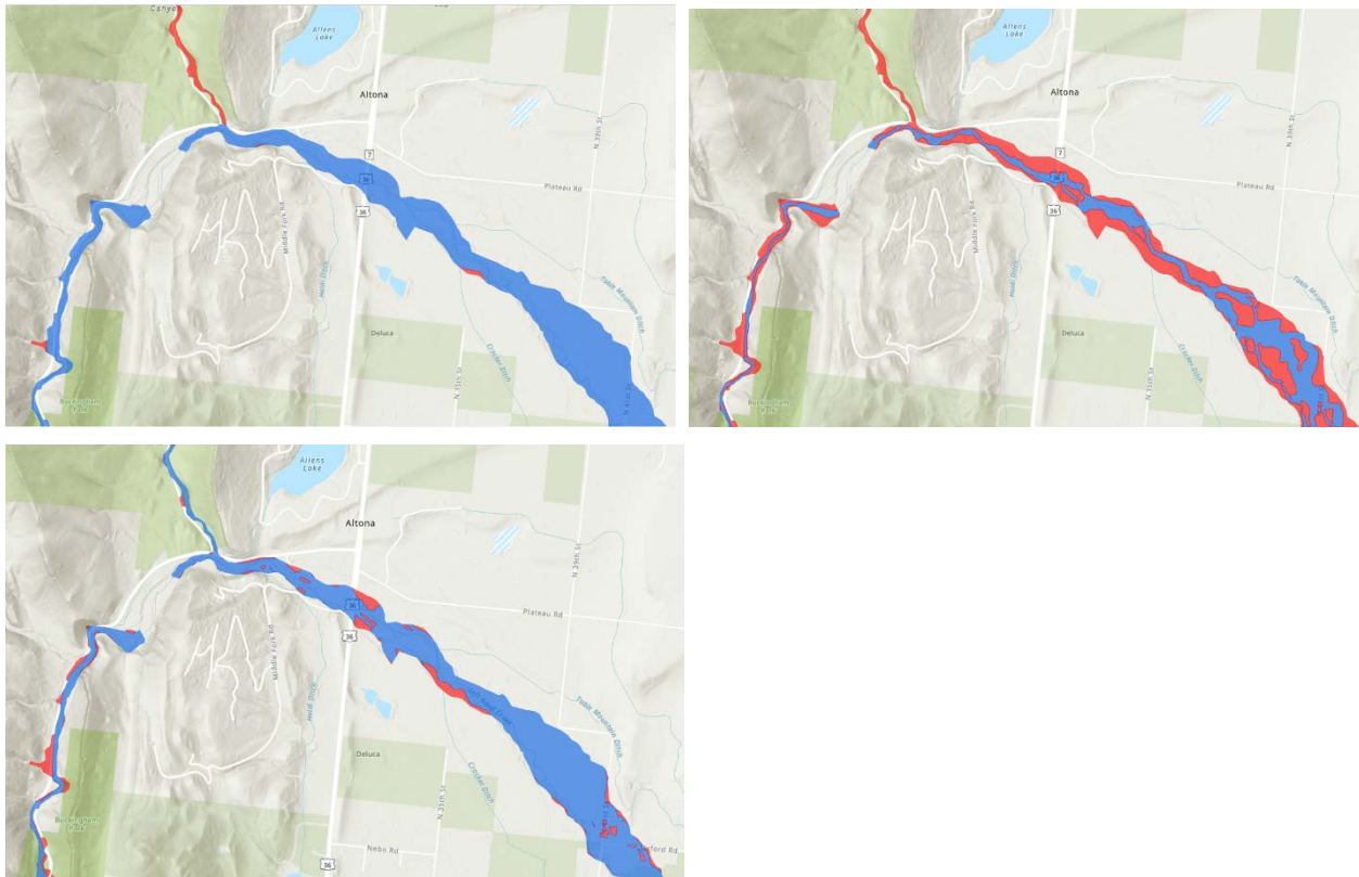
Figure 1. Comparisons of flood risk delineations along Left Hand Creek, with “hits” (blue) and “misses” (red) compared against 2013 flood inundation along Left Hand Creek A) FHZ, B) Floodway, and C) combined 100-year floodplain (combining 2013 and preliminary 2019 FIRMs). Note that 2013 flood inundation extent data was missing for one large stream segment, which is the cause for the large gap in each image.
