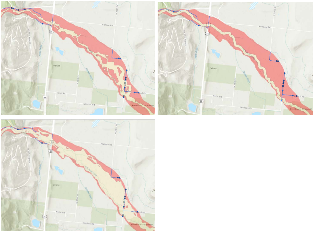
Figure 4. County infrastructure (bridges, culverts, and roads) located along Left Hand Creek in the FHZ (infrastructure in dark blue, zone in red) compared to infrastructure located in various regulatory zones (infrastructure in light blue, zone in light yellow). A) Floodway, B) 100-foot setbacks, C) combined 100-year floodplain.
