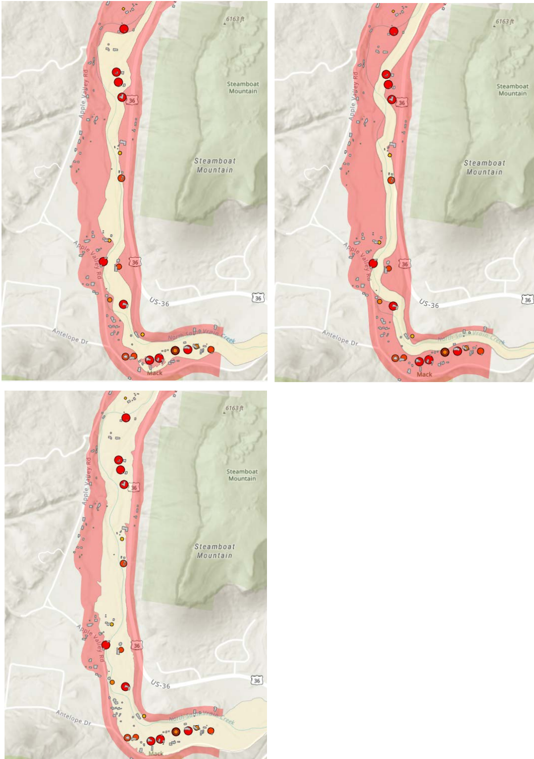
Figure 6. Damage estimates from the 2013 floods along North Saint Vrain Creek, with larger redder points meaning more complete damage and smaller orange and yellow points meaning less damage. The damage estimates are shown overlaid with the various regulatory zones (light yellow) and the wider FHZ (light red). All building footprints in the FHZ are shown in light grey. A) Floodway, B) 100-foot setbacks, C) combined 100-year floodplain.
