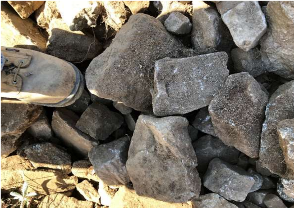
Photograph 5: Typical rockfill encountered in TP-103.
