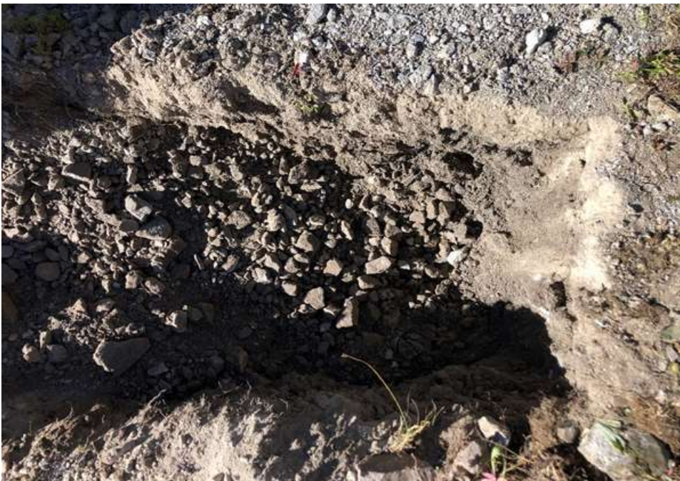
Photograph 4: Fill encountered in TP-102.
