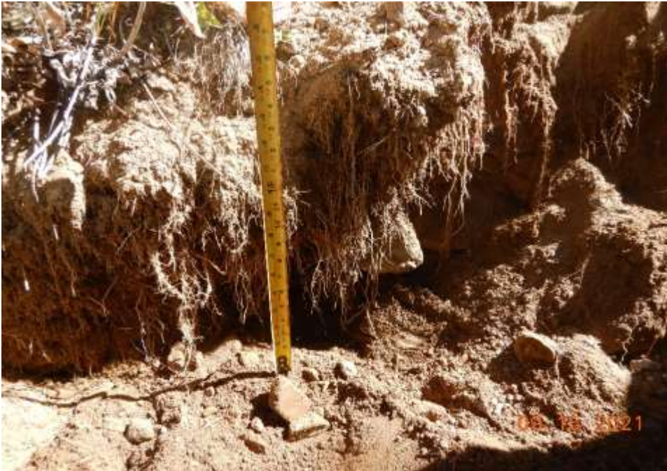
Photograph 1: Excavation of TP-101. Roots from vegetation extended approximately 1 foot into the earth fill.
