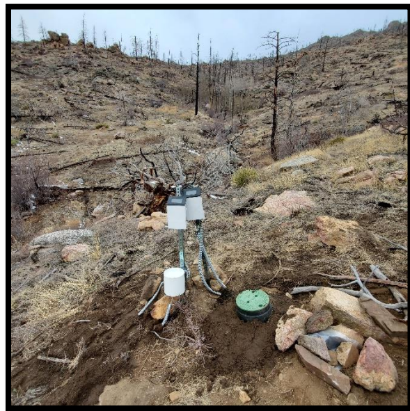
Figure 6: Monitoring station with rain gauge and data loggers visible.
