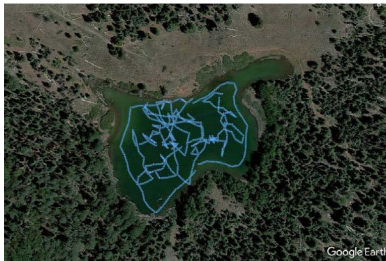
Figure 2. Nine depth tracks were run on Hack Lake and combined with a track of the wetted perimeter on September 22, 2021, projected in Google Earth.
