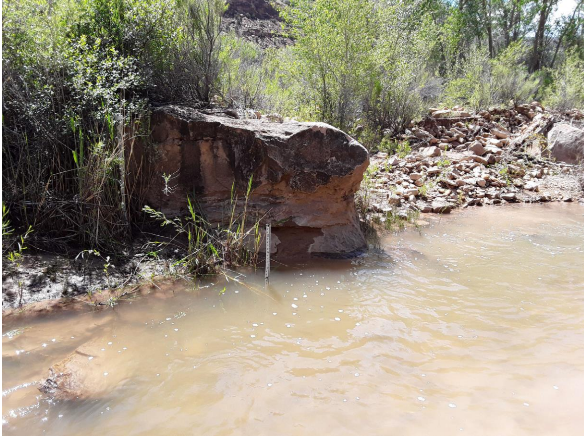
Gage installation (6/19/2019). Onset Hobo MX2001 pressure transducer located at foot of staff gage in center of photo. Cable buried in conduit in bank to vertical pvc pipe behind bush on left edge of large boulder. Right side of photo is upstream.
