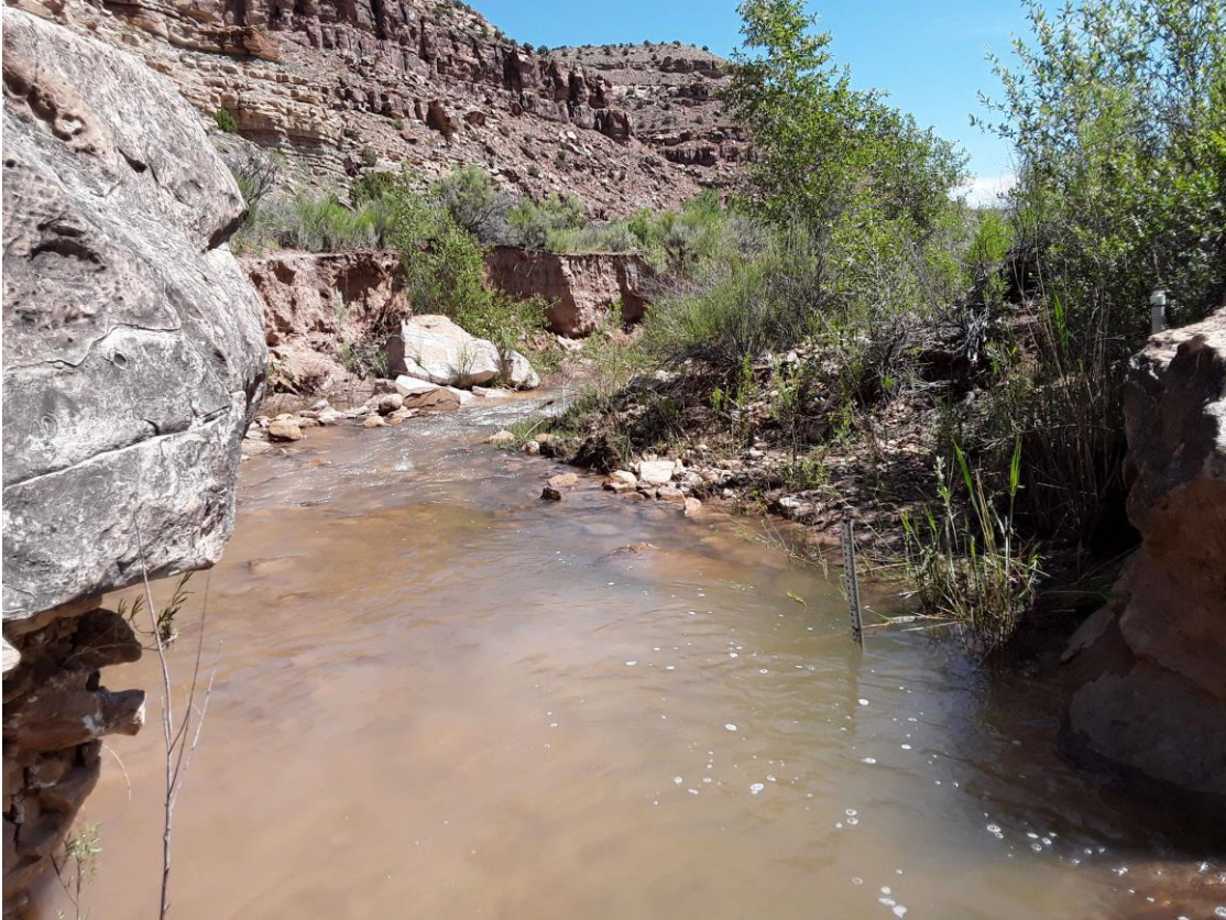
Control looking downstream on 6/19/2019. Staff gage is on right bank, right edge of photo. Standing between the two large boulders that form gage pool and constrict flow, looking downstream at control.
