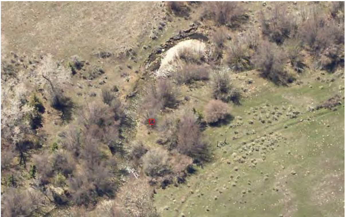
Figure 6-13 EagleView imagery of the Fox Ditch Diversion Dam. Notice sediment deposition in the upper third of the photo.
