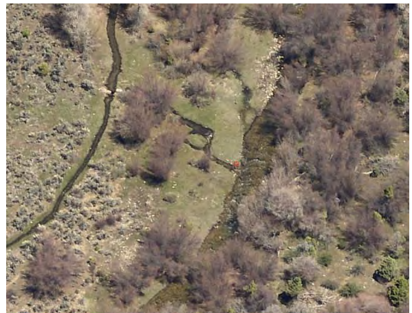
Figure 6-11 Flow returns from excess diversion.
