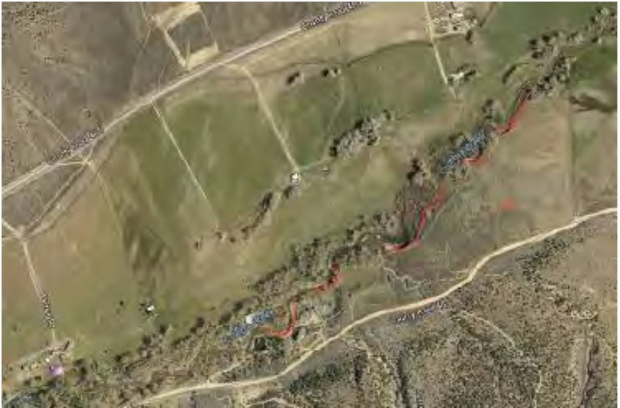
Figure 4-24 Areas where Culebra Creek is cutting into high terrace above Sanchez Canal.
