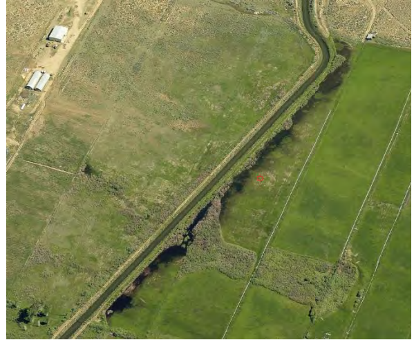
Figure 6-60 Canal causing backwater right floodplain San Francisco Creek drainage.
