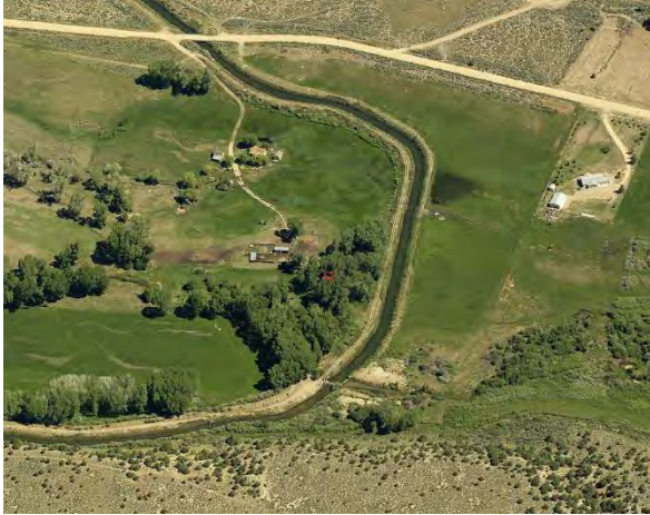
Figure 6-59 Backwater from canal embankment right edge of floodplain Vallejos Creek.
