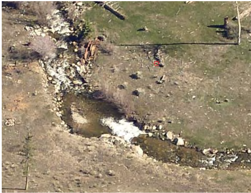
Figure 6-26 Stream stabilization structures near Canon Ditch No. 1. Note structure is placed backward, with the furthest downstream point occurring in the middle of the structure.
