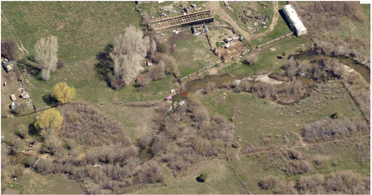
Figure 6-18 Antonio Sanchez diversion structure, sediment deposition as mid-channel bars observed above the structure along with bank erosion. Structures present in floodplain. EagleView Connect Explorer – May 13, 2019
