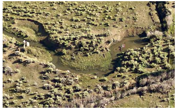
Figure 6-82 Bank erosion along San Acacio ditch.
