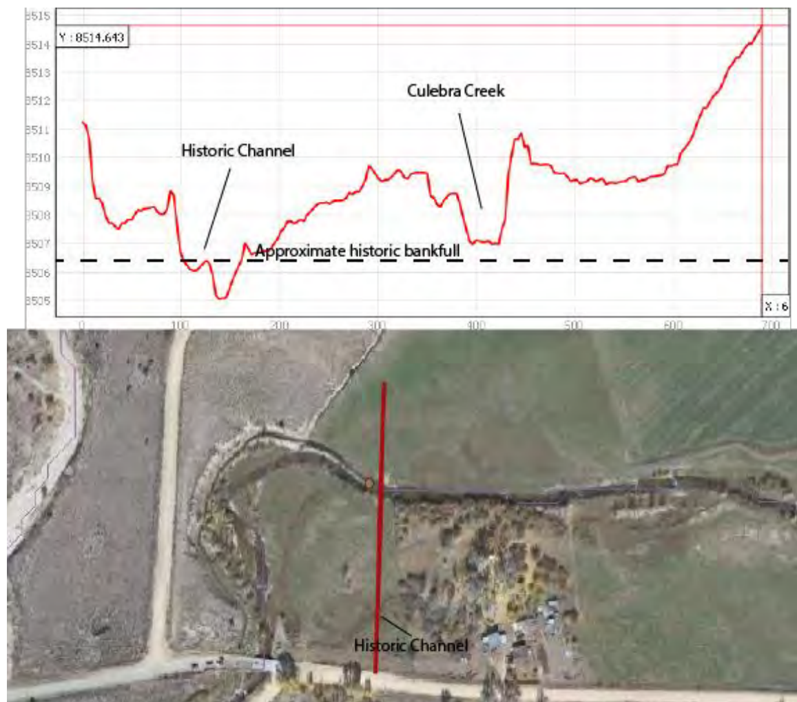
Figure 6-20 Guadalupe Sanchez 2011 Lidar profile. The present-day Culebra Creek channel is approximately two feet higher than the historic channel and wider than the historic channel (approximately 32 ft vs 55 ft).
