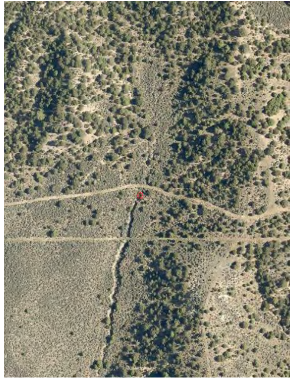
Figure 16-4 Road concentrating flows resulting in headcutting below road 37.141870, -105.318386, Eagleview aerial imagery dated May 13, 2019
