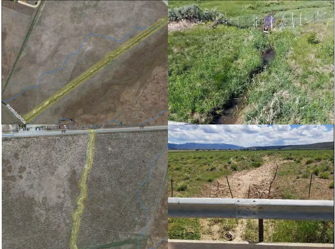
Figure 4-55 Top Left aerial view Return flow channel, Cerro Ditch and Rito Seco historic alluvial channel (26), notice channel pattern and signs of deposition on floodplain. Top right Unknown (26) view from the road, notice channel incision. Bottom Left aerial view of Rito Seco historic alluvial channel (24) notice channel pattern and aggradation. Bottom Right (reach 24) aggradation in channel apparent from the road.
