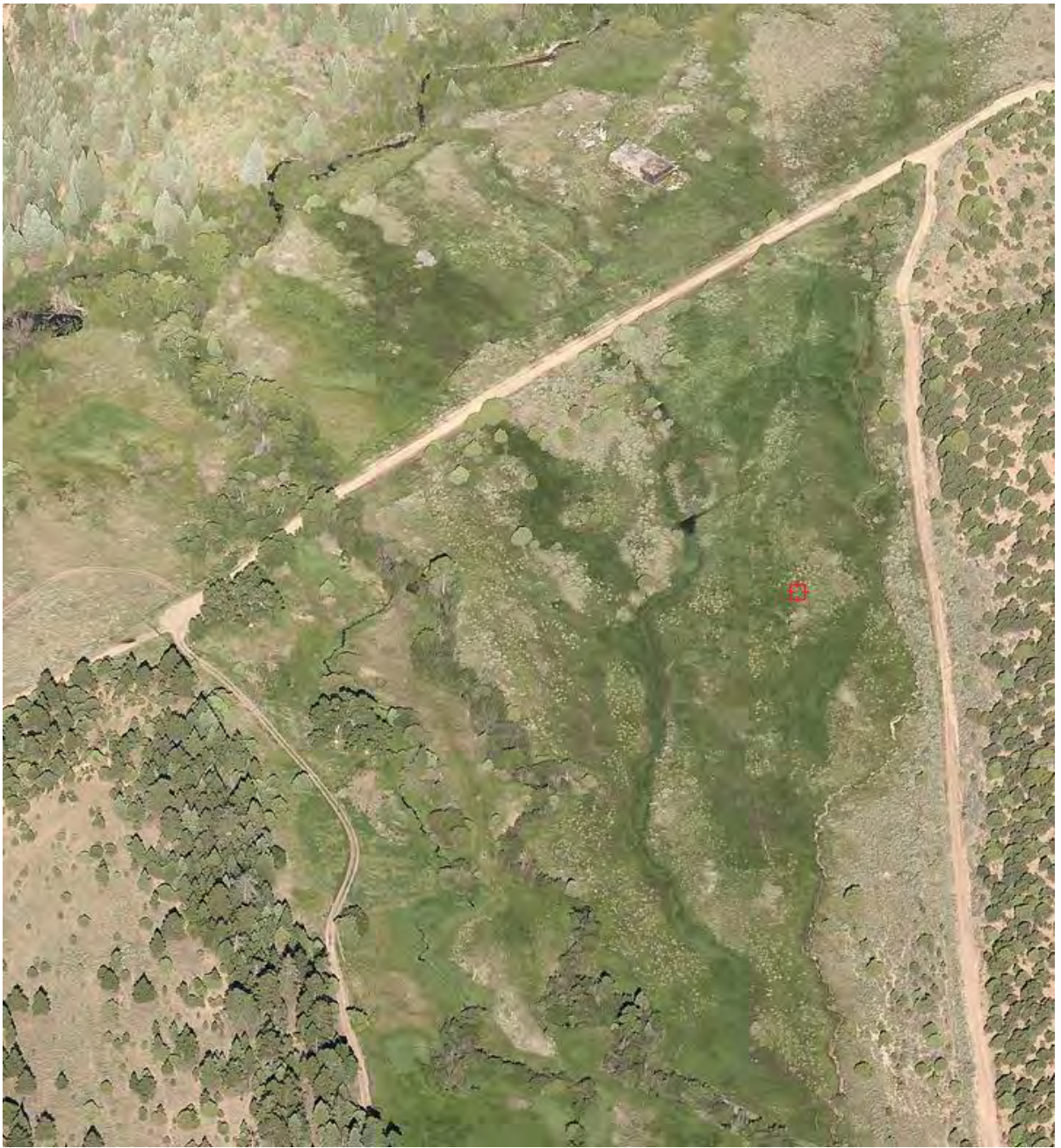
Figure 6-102 Channel braiding in Alamosito Creek alluvial fan. Channel braiding reduces stream energy and allows sediments to be deposited.
