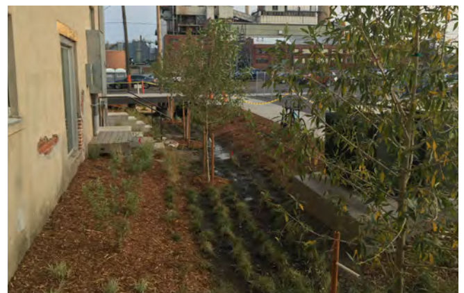
A rain garden next to STEAM on the Platte, near West Colfax Avenue and the South Platte River. The rain garden allows stormwater runoff to infiltrate into the ground where sediment and pollutants are removed prior to discharging to the South Platte River.
