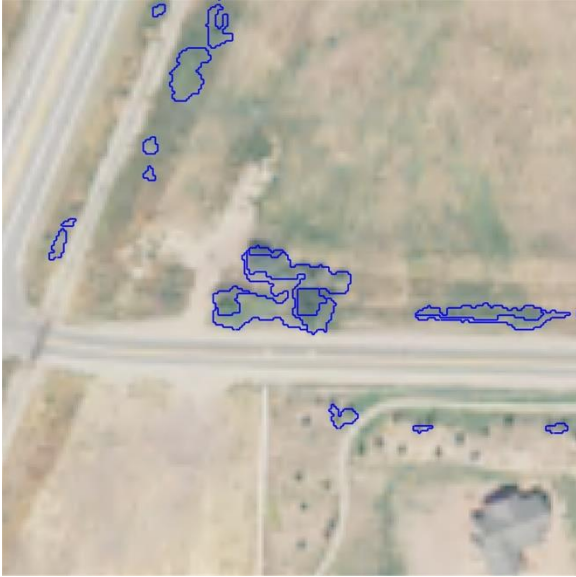
Figure 14 Canopy segmentation using the multi-resolution segmentation algorithm (scale = 25, shape = 0.1, compactness = 0.5). Objects are spectrally grouped, causing other classes to be grouped with RO.
