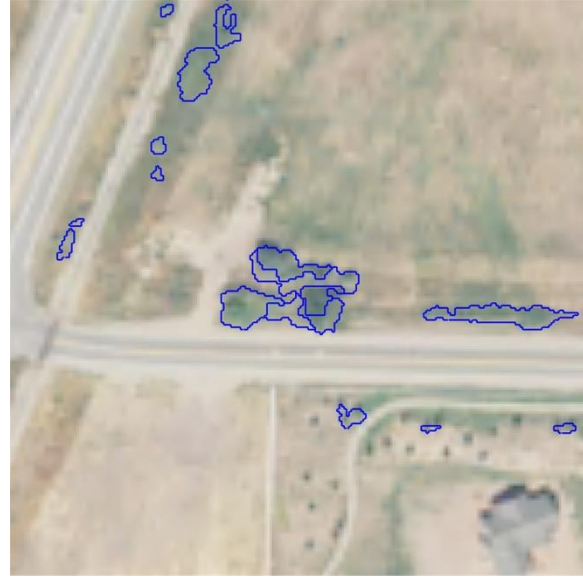
Figure 15 Canopy segmentation using the multi-resolution segmentation algorithm (scale = 25, shape = 0.4, compactness = 0.5). Shaded and bright areas occupy their own objects regardless of if the areas represent the same tree.
