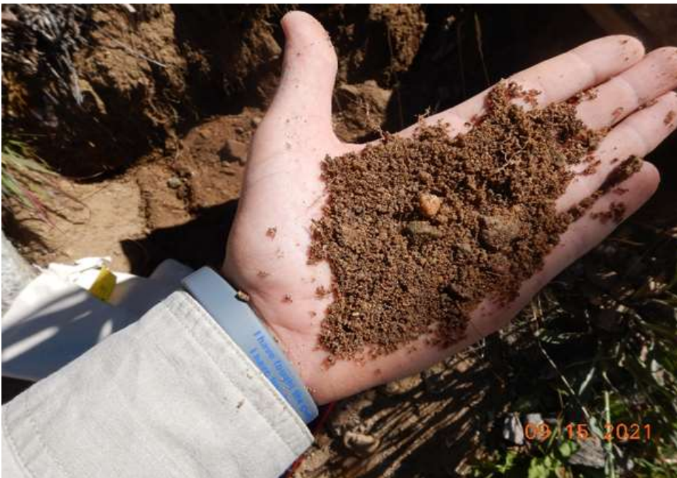
Photograph 2: Typical finer material encountered in TP-101. Poorly graded sand with gravel.
