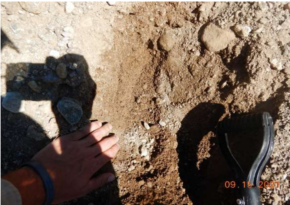
Photograph 6: Soil on the west side of the reservoir sediment stockpile. Well graded sand with silt and gravel.
