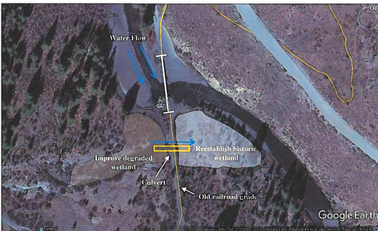
Map 2: Alignment of the new, 100' bridge, the relief culvert and improved/re-established wetlands. Water flow direction shown with blue arrows.
