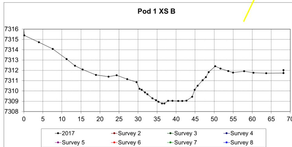
Example plot of station-elevation data from XS1b on West Creek at Glen Haven (above). These data are stored in a file with photos (right) that is prepared to overlay additional surveys. The original point data and field notes are recorded separately.
