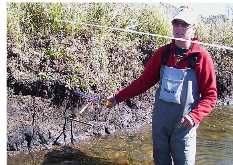
Measuring accretion on a set of bank pins
