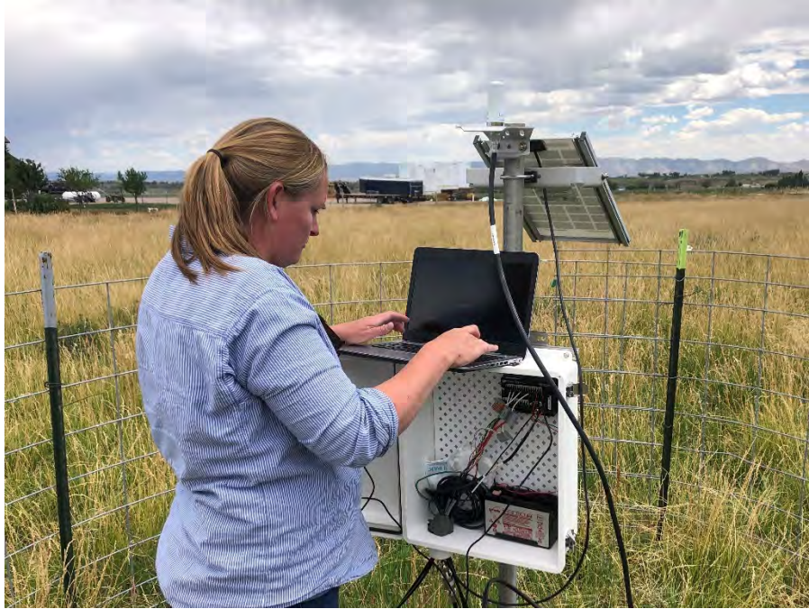
Downloading soil moisture data from the data logger
