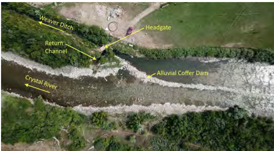
Image 3-1 Alluvium dam, boulder grade control, concrete headgate structure, and the beginning of the Weaver Ditch.
