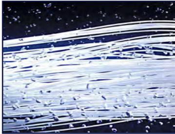
ZeeWeed water treatment is a process technology that produces high quality treated water by filtering water through SUEZ Water Technologies & Solutions' proprietary and patented immersed ZeeWeed ultrafiltration membranes. ZeeWeed 1000 series membrane utilize "Outside-In" flow through a hollow-fiber membrane. The small pore size of the ultrafiltration membrane excludes particulate matter from the treated water.
