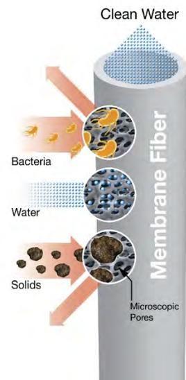
**ZeeWeed® UF membranes operate under gravity, drawing clean water to the inside of the membrane fiber (outside-in flow path), while keeping impurities out.**
