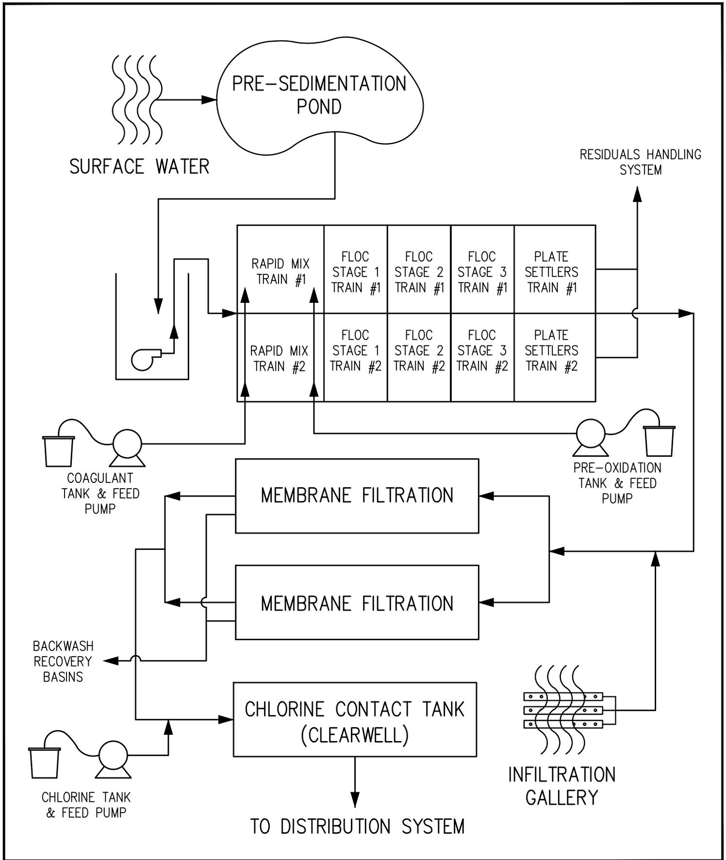
**FIGURE 13 - SURFACE WATER PROPOSED PFD**
