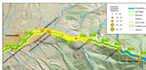
Figure 2-2. Late season streamflow observed on the Crystal River in the late summer of 2011. Green callouts indicate measured flows. The thickness of the blue and yellow lines indicate the relative magnitudes of observed flows and the CWCBS Instream Flow Right
