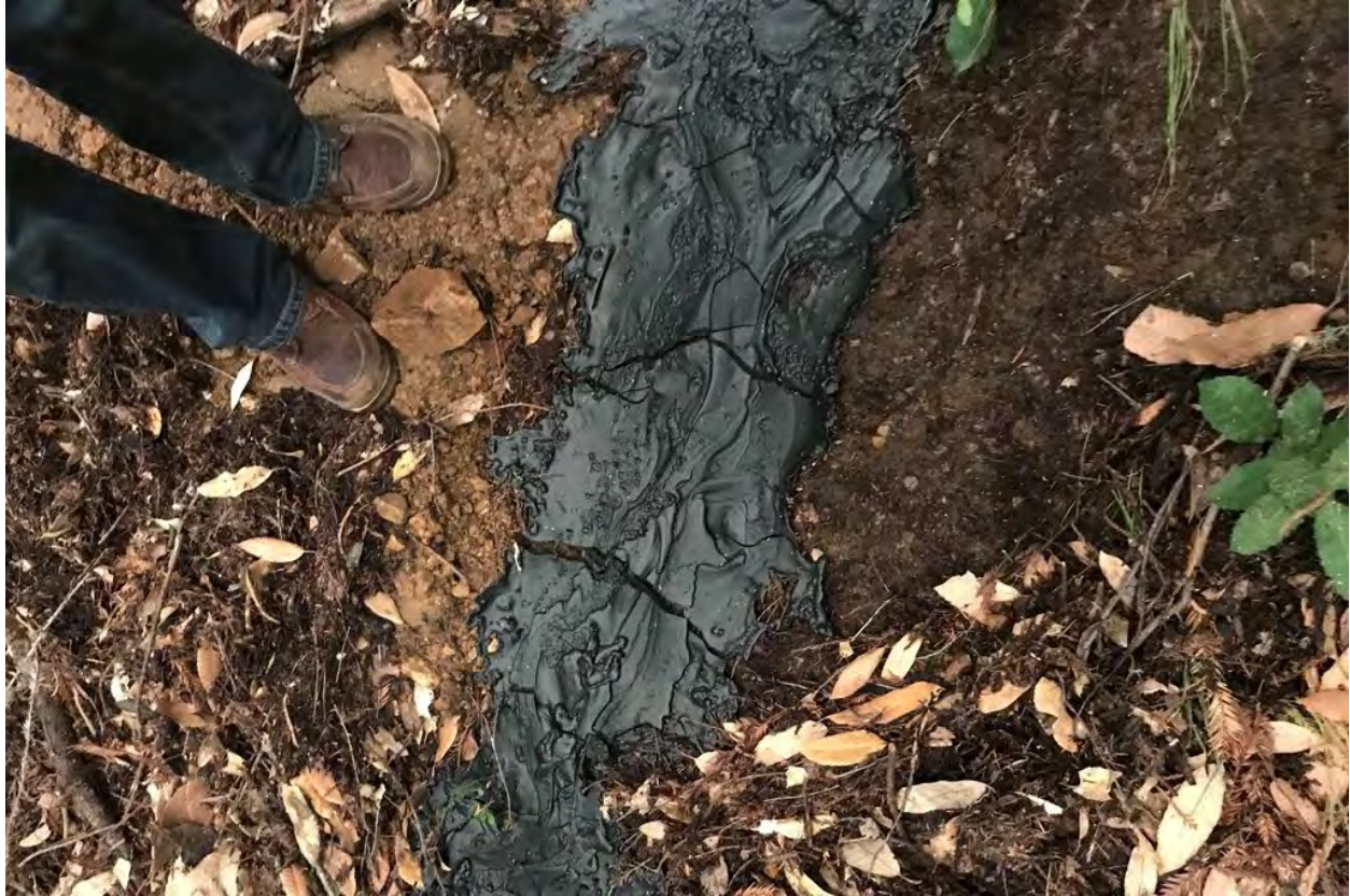
A melted high density polyethylene water pipe burned in a 2020 fire in the San Lorenzo Valley, CA. Credit: James Furtado/San Lorenzo Valley Water District
