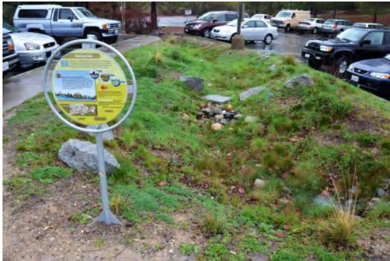
In Nevada City, California, a rain garden is used to catch rainwater runoff from parking lots and allow the water to sink into the ground. Photo: Jacob Dyste.
