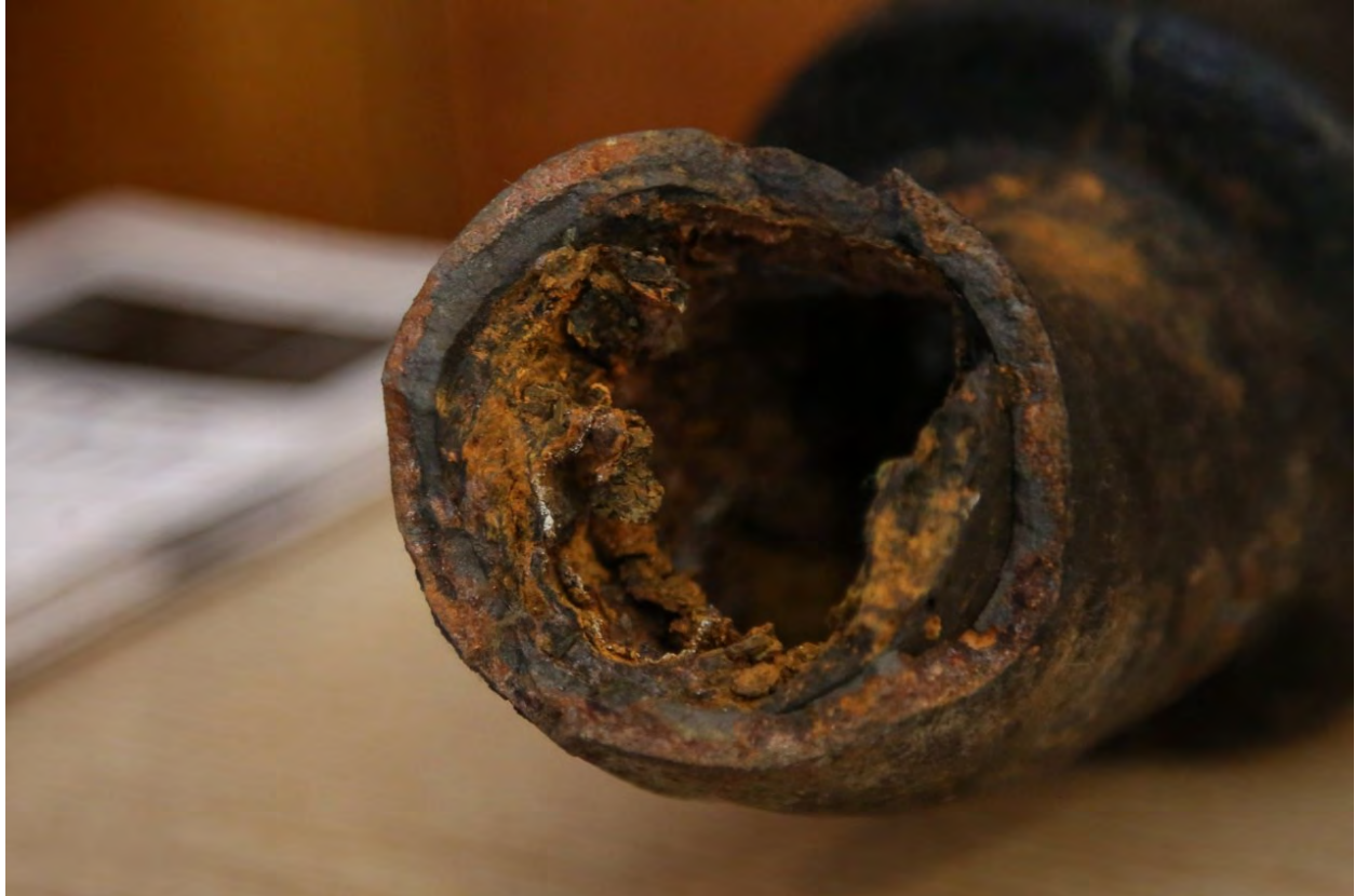
A corroded pipe a Flint, Michigan, resident removed from her home. PHOTO: KIMBERLY P. MITCHELL/ZUMA PRESS
