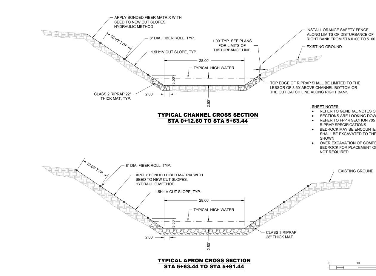
REFER TO GENERAL NOTES ON G0-04 SECTIONS ARE LOOKING DOWN STREAM REFER TO FP-14 SECTION 705 FOR BEDROCK MAY BE ENCOUNTERED AND SHALL BE EXCAVATED TO THE LIMITS
