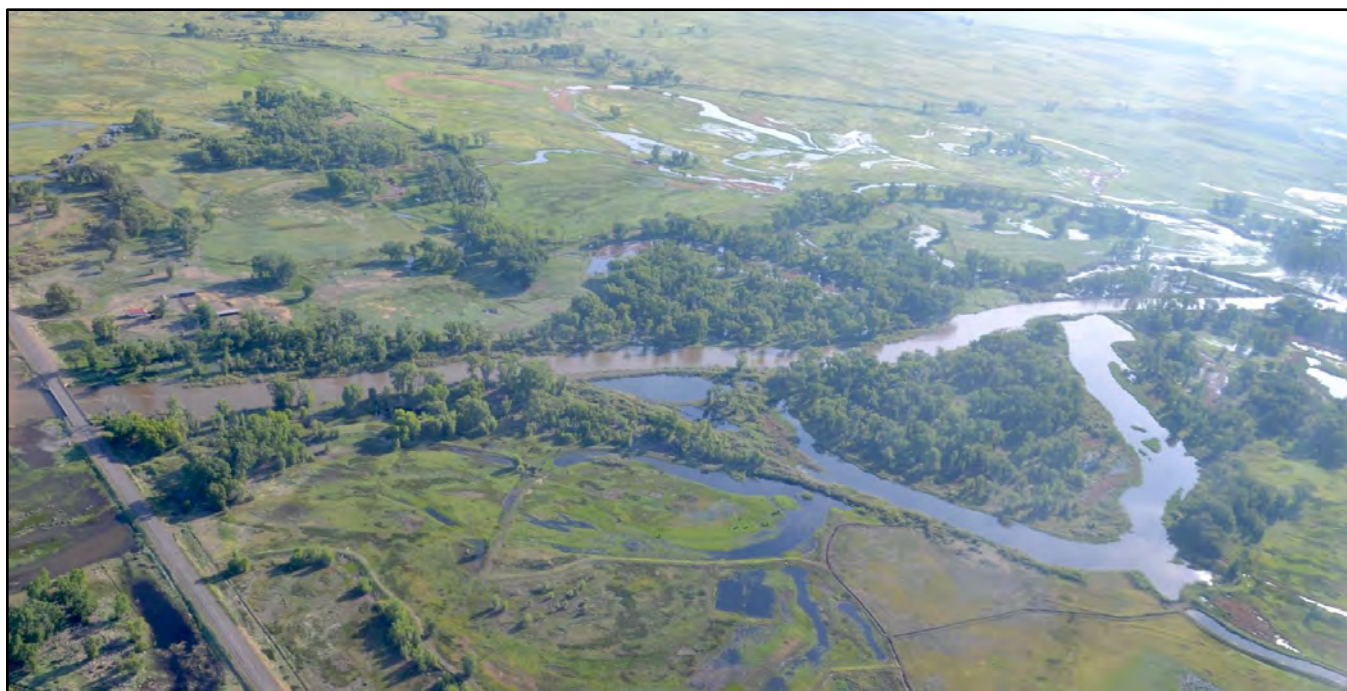
Figure 2.14: Channelization of the Rio Grande at the Soldiers Home Road (County Road 3E).
