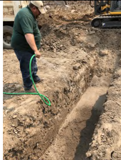
Photo 2. Moisture conditioning filter sand for Test #2. Note color variation between wet and dry sand.
