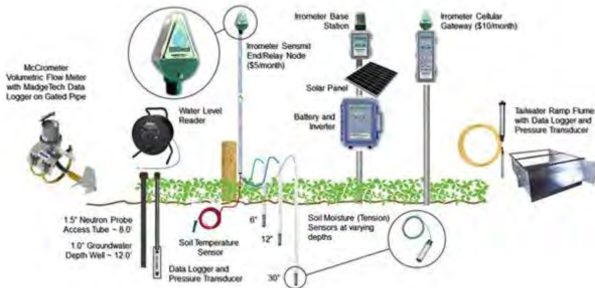
Figure 2.2: Instrumentation for Irrigation Evaluation Sites
