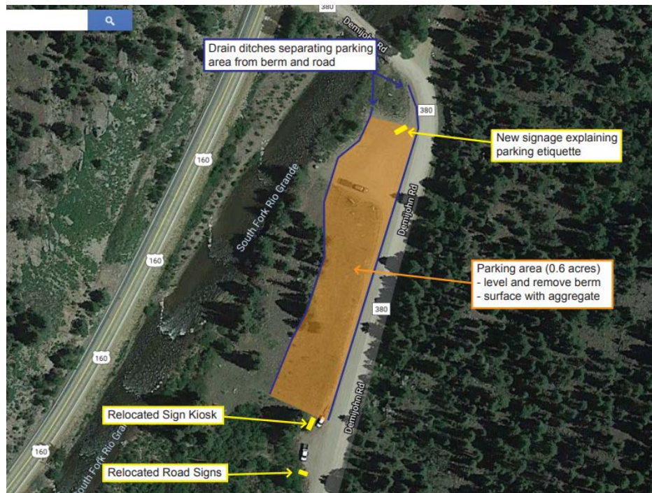
Figure 3. OHV Unloading and Parking Area Design
