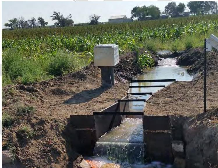
Flumes were installed according to Colorado Division of Water Resources publication “Standard Operating Procedures: Discharge Measurement at Parshall Flumes.” Flume measurement accuracy was checked using a USGS Pygmy Current Meter in combination with AquaCalc Pro Plus Stream Flow Computer (JBS Instruments).
