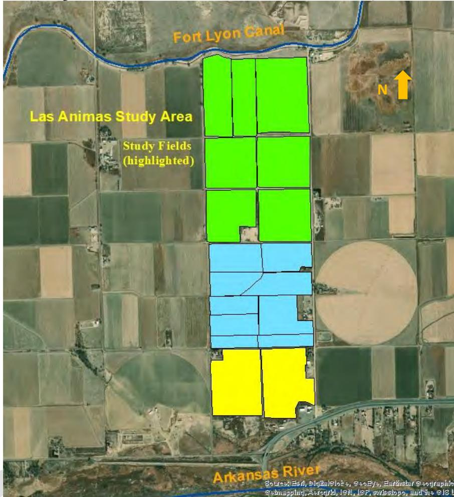
Irrigation supply for the Las Animas study area is diverted from the Fort Lyon Canal through two headgates approximately 2 miles north of the Arkansas River at Las Animas. Tailwater ditches carry any tailwater return flows, groundwater seep, and precipitation runoff back to the Arkansas River.
