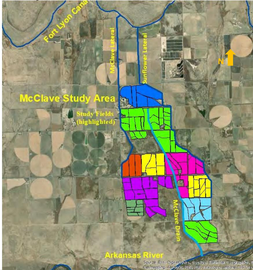
Irrigation supply for the McClave study area is diverted from the Fort Lyon Canal through two lateral ditches – the McClave Lateral and the Sunflower Lateral – which follow ridge lines on the western and eastern boundaries of the study area respectively. The McClave Drain channel dissects the study area from north to south and carries any tailwater return flows, groundwater seep, and precipitation runoff back to the Arkansas River.
