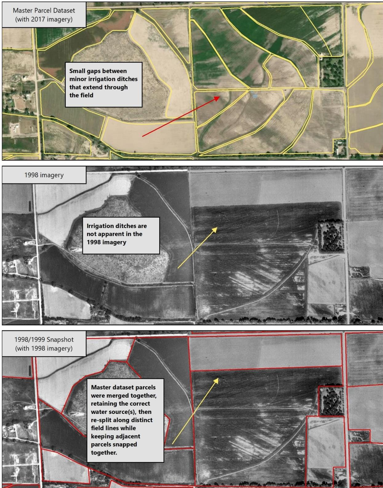
Figure 4 – This area is north and west of Lamar within the HIM area. It displays the process of removing gaps between minor laterals.
