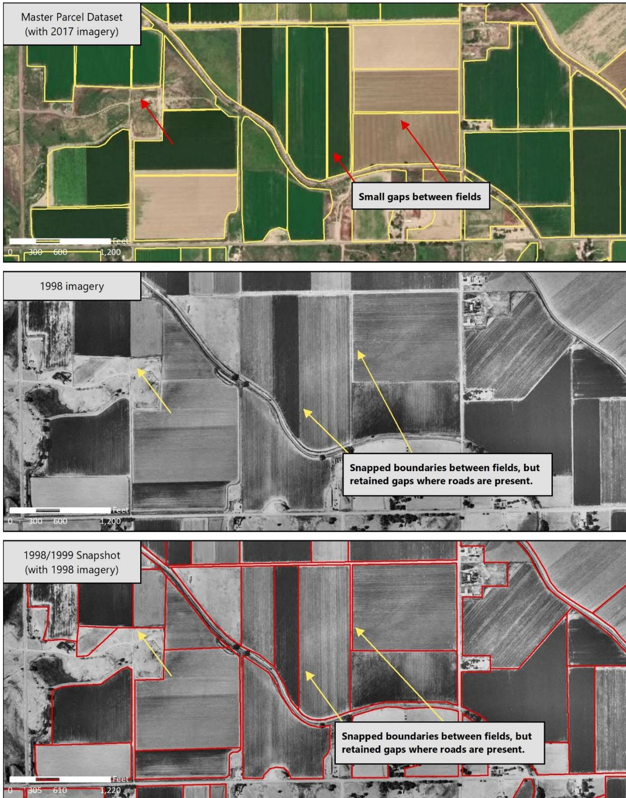
Figure 3 – This area is just southeast of Rocky Ford within the HIM area. It displays the process of snapping adjacent parcels where no road exists.
