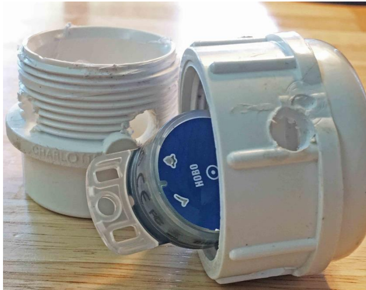
1. Temperature sensor in a protective PVC case made from plumbing fittings
