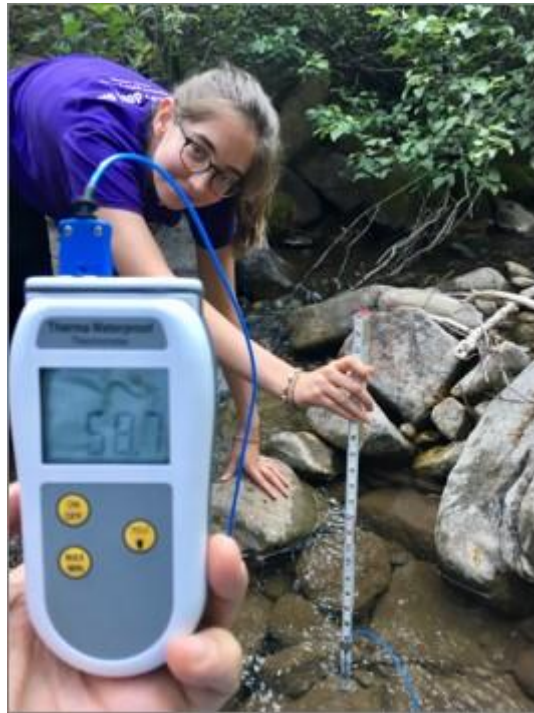
3. Testing for variations in tributary water temperature using a hand-held sensor
