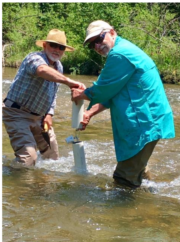
2. Installing a PVC case with sensor at riffles in the main stem, using two weights to secure the placement
