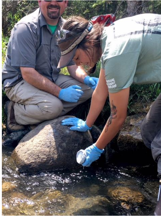
5. Installation at the lowest Slate site using epoxy to attach the PVC case with sensor
