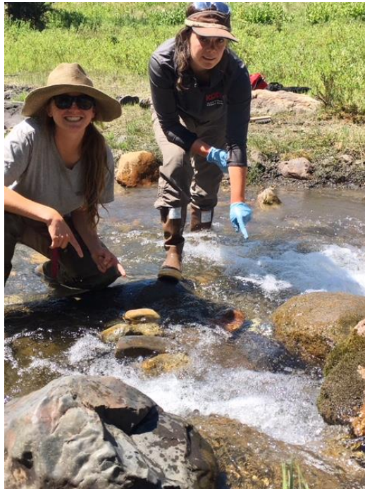
6. Installation with two methods at the highest Slate site, for comparison, one using a portable mesh bag with rocks and a PVC sensor case and the other using epoxy to attach a PVC case
