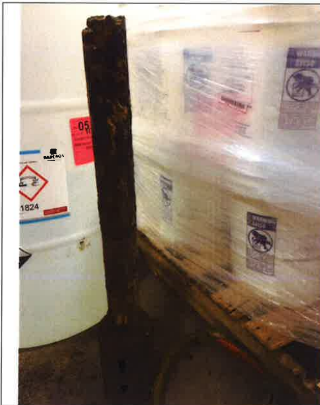
Photo 33: Piece of gate stem and coupler removed from upstream gate assembly. Date: 03-21-2019 Source: G. Jeffrey (Evergreen Metro)
