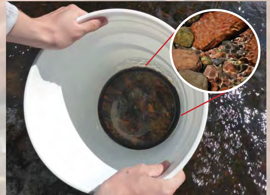
This simple tool — a 5 gallon bucket with plexiglass bottom — allows researchers to study stream beds (without sticking their heads underwater!).
