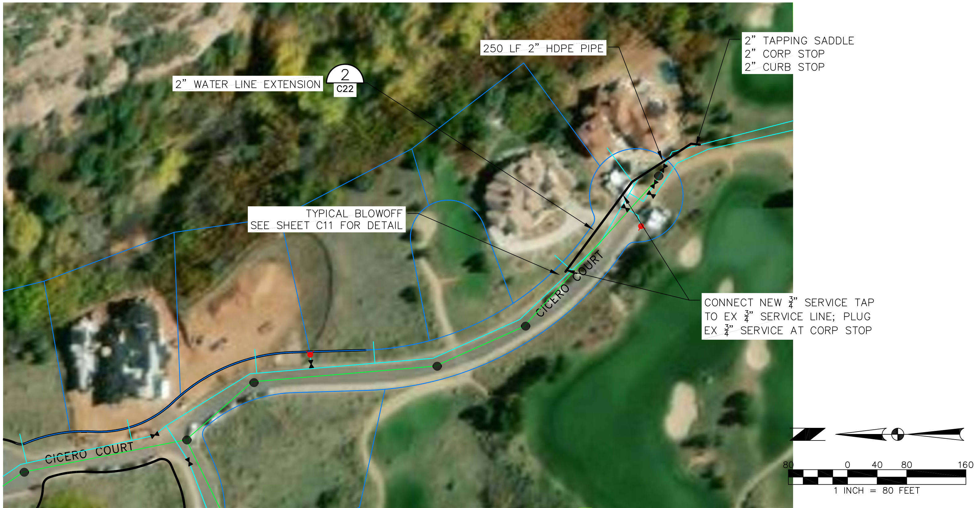
2" WATER LINE EXTENSION SCALE: 1" = 80'
