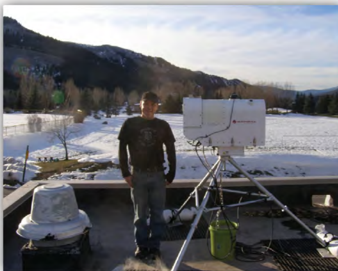
Figure 8. CWCB Radiometer Installed in CCMRB Program Target Area for 2014-15 Winter Season (Courtesy CWCB)
