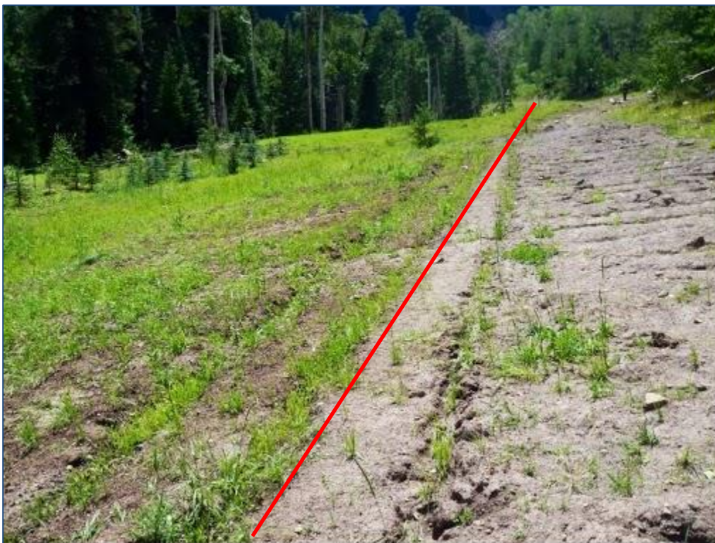
Figure 33. Contrast between alluvial fan area amended with compost-biochar (left of red line) and without (control-right of red line). September 24, 2013.
