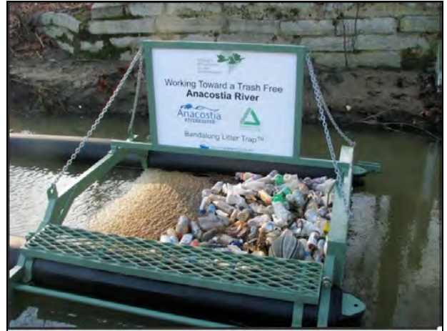
Figure 5 : Bandalong Litter Trap in Washington DC
